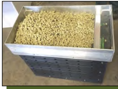
Refilling tray on cartridge with bulk media.
